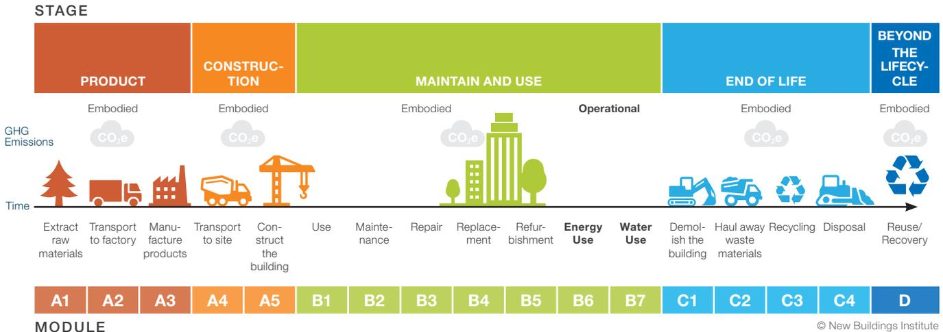
Most LCAs, WBLCAs, and EPDs focus on stages A1-A3: the extraction of raw materials, transport to the factory, and manufacturing of the products. Stage A has the biggest potential for embodied carbon reduction.
