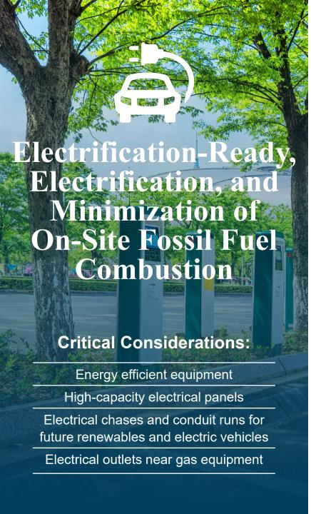
Carbon neutral buildings minimize or eliminate on-site natural gas and other fossil fuels because fossil fuel combustion (i.e., propane and gas) directly contributes to GHG emissions. Building electrification combined with energy efficiency can reduce air pollution, assist with better grid management, and permanently lower utility expenses.
