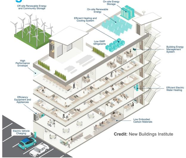
Additional components of net zero energy building versus carbon neutral buildings
