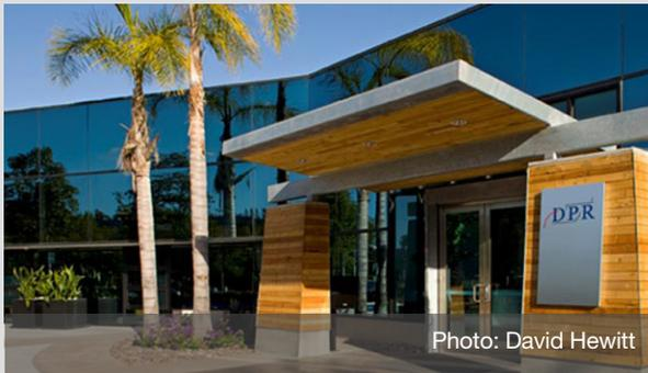
Taking advantage of San Diego's mild climate, the DPR Construction office building was designed to use cross and stack ventilation strategies to passively ventilate and cool the open office area. By installing operable windows at the north curtain wall and roof monitors at the south side, the number of hours the HVAC system is used was reduced by 79% a year.
