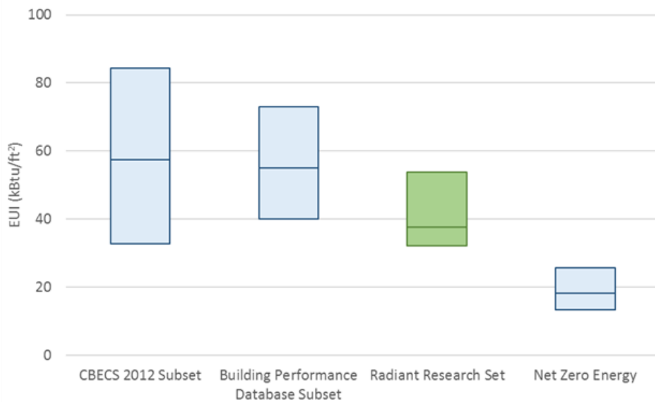
Figure 5: Box plot bounding 25 th and 50 th percentile EUI of the research set and various benchmarks
